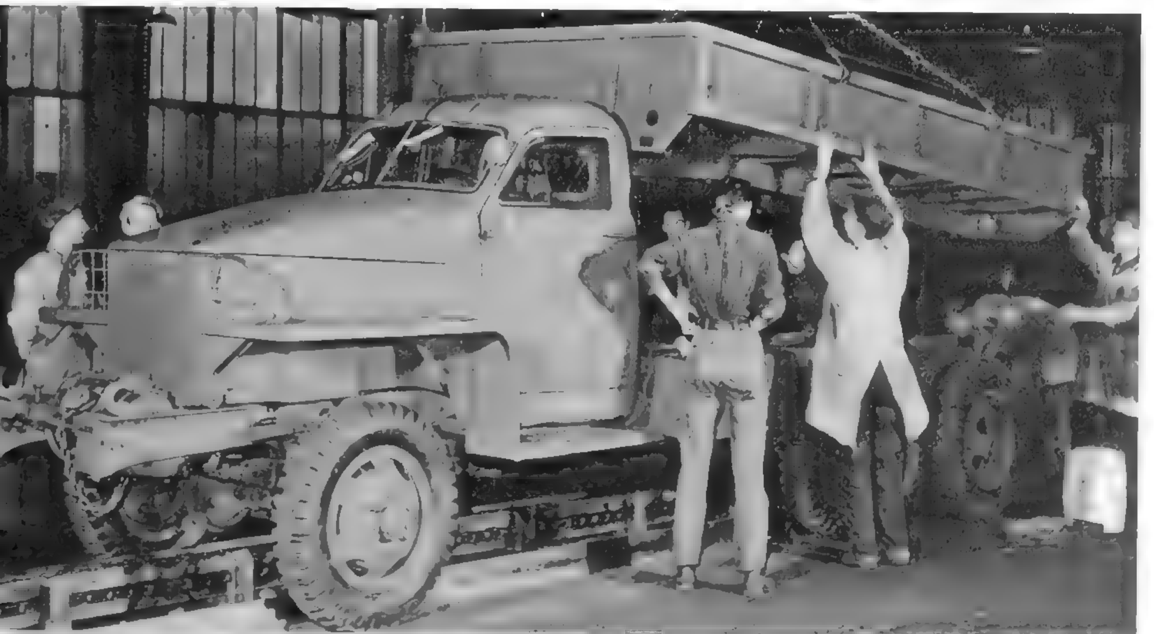
The vast majority of the US6 models were all-wheel-drive cargo trucks like this one. This vehicle is having its bed mounted in Studebaker's downtown South Bend, Indiana, plant. This is an early production truck, as is evidenced by the Studebaker nameplate on the grille. (Photo courtesy of Bryce Underlin collection)
